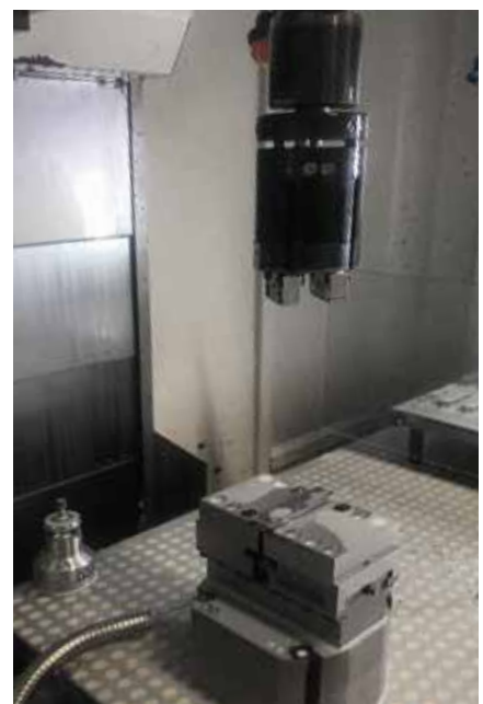
Pneumatischer Zentrischspanner PZS 180-80 AT Pneumatic centre-clamping vise PZS 180-80 AT
